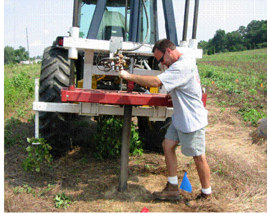
Figure B 2.11 Soil core sampler for bulk density and soil moisture determination on the Pacolet sandy loam soil near the Old Rotation Experimental Plots of the Auburn University and USDA-AR Surface soil
