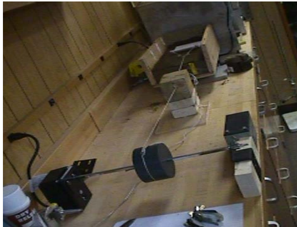
Figure A 2.3 Soil cone penetration reading using Sintech/2G at the USDA-ARS- NSDL facility in Auburn, AL precision farming lab.
