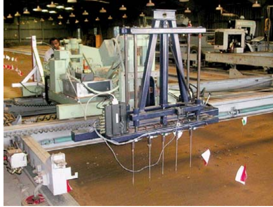
Figure B 2.6 Soil cone penetration reading using multiple-probe soil cone penetrometer on the Norfolk sandy loam soil bin at the USDA-ARS- NSDL facility in Auburn, AL.
