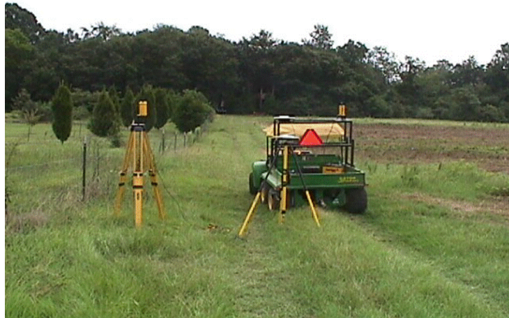
Figure B 2.10 A dual-frequency RTK, AgGPS ® 214, GPS receiver ( cm level accuracy) with ground station for digital elevation data acquisition on Pacolet sandy loam soil near the Old Rotation Experimental Plots of the Auburn University and USDA-ARS- NSDL in Auburn, AL.
