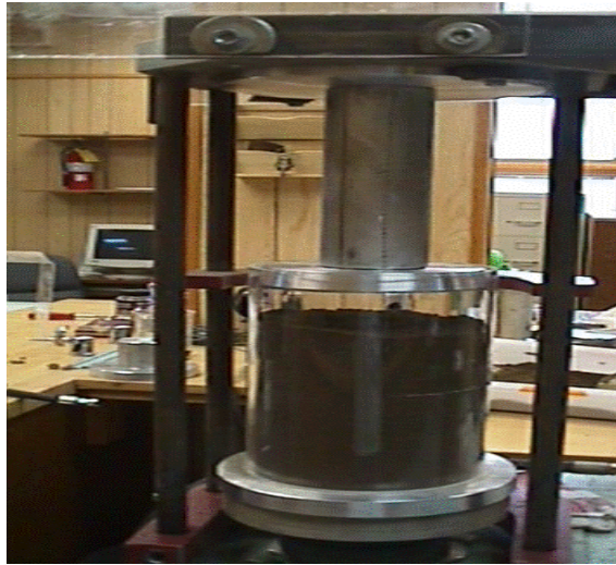
Figure B 2.1. Soil compression in the USDA-ARS NSDL facility in Auburn, AL precision farming lab.
